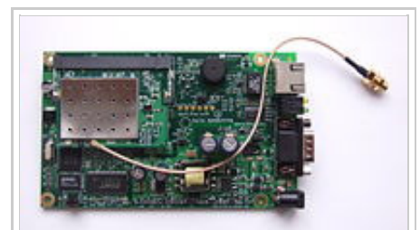
An embedded RouterBoard 112 with U.FL-RSMA pigtail and R52 mini PCI Wi-Fi card widely used by wireless Internet service providers (WISPs) in the Czech Republic.
