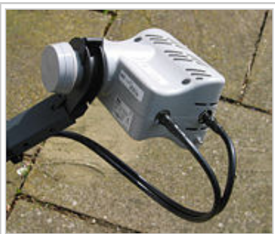
The two-way "iLNB" used on the ASTRA2Connect.
